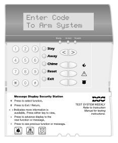
The **Liquid Crystal Display** (LCD) displays prompts and system information on two 16 character lines.
